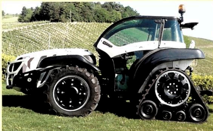
SkyJump's Dualsteer system combines central chassis articulation with the front turning wheels to achieve a 60-degree turning angle
