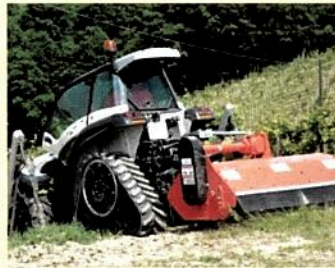
The Cat I/II rear linkage lifts 2700kg and hydraulic flow of 28.5 lit/min is available for attached implements
